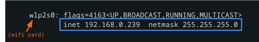
ip address identifies a device subnet mask indicates the whole network's size
